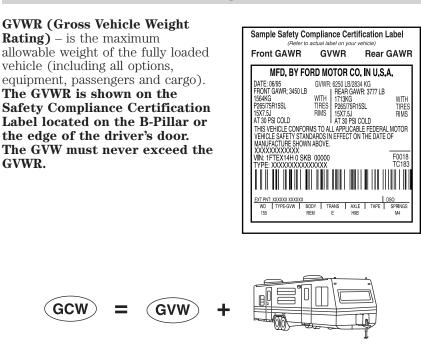
**GCW (Gross Combined Weight)** – is the weight of the loaded vehicle (GVW) plus the weight of the fully loaded trailer.
